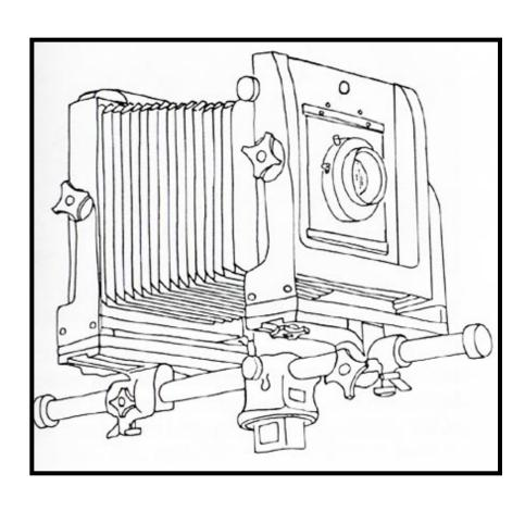
Built like an accordion, with a lens in the front, a viewing screen in the back, and flexible bellows in between.
